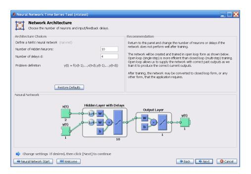
The standard NARX network is a two-layer feedforward network, with a sigmoid transfer function in the hidden layer and a linear transfer function in the output layer. This network also uses tapped delay lines to store previous values of the x(t) and y(t) sequences. Note that the output of the NARX network, y(t), is fed back to the input of the network (through delays), since y(t) is a function of y(t - 1), y(t - 2), ..., y(t - d). However, for efficient training this feedback loop can be opened.
