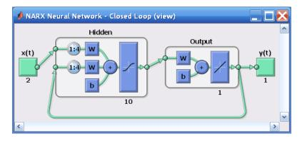
**10** Remove a delay from the network, to get the prediction one time step early.
